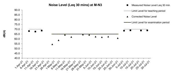
Remark: Corrected Noise Level was applied on 29 April 2021; 5, 11, 17 and 28 May 2021; 3, 9, 15, 21, and 30 June 2021; Corrected Noise Level = Measured Noise Level - Baseline Noise Level (i.e. 67.7 dB(A))
